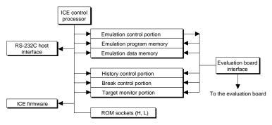
Fig. 2.3.1.1 Block diagram of ICE functions
